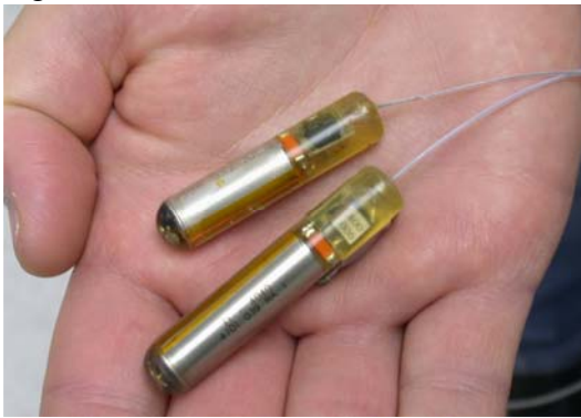
Figure 7. Pulse coded radio transmitter
